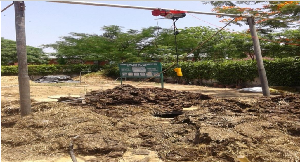
Fig. 4: Semi-automatic solid bio-digested slurry removal machine with lifted bio-digested slurry
