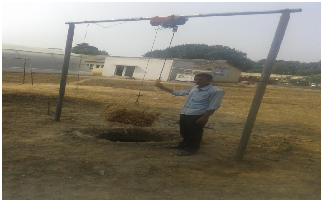
Fig. 5: Bales lifted by Semi-automatic solid bio-digested slurry lifting machine
